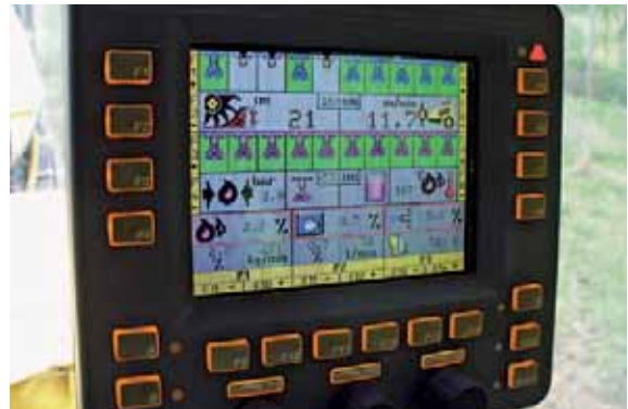
Process control by dosing computer.
