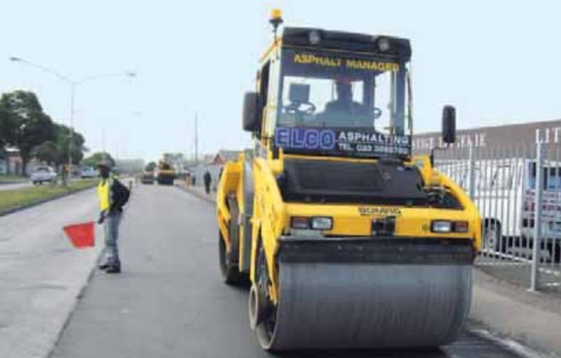
Fig. 2: BW 151 AD-AM; 9 t operating weight together with 1.680 mm working width.
