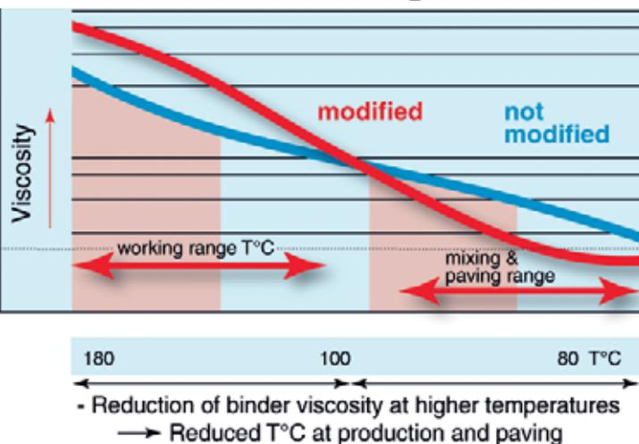
Fig. 8: How WMA additives influence the compactability (Source: German asphalt association).
