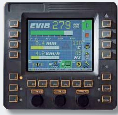
Fig. 3: Bomag ASPHALT MANAGER provides target values for compaction.
