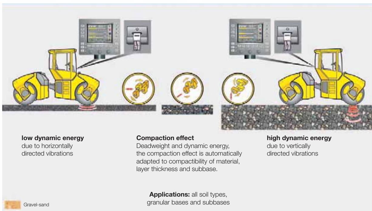
Fig. 1: Automatic optimisation of compaction: one solution for all applications.
