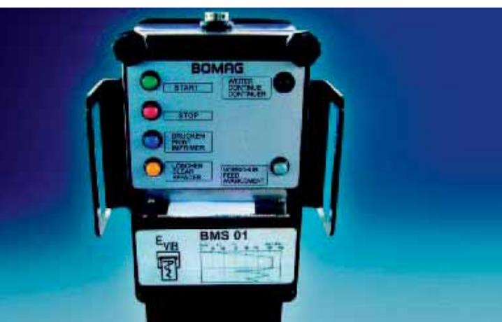
Fig. 9: Proof rolling at site: Print-out of  $E_{VIB}$  and T°C.
