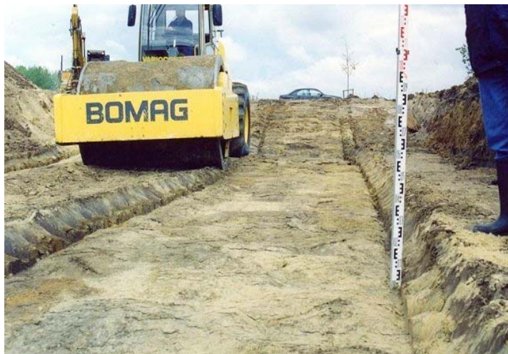
Fig. 7: View of the test and the depression of the surface after 8 passes with the BW 225 D-3 BVC with polygonal drum
